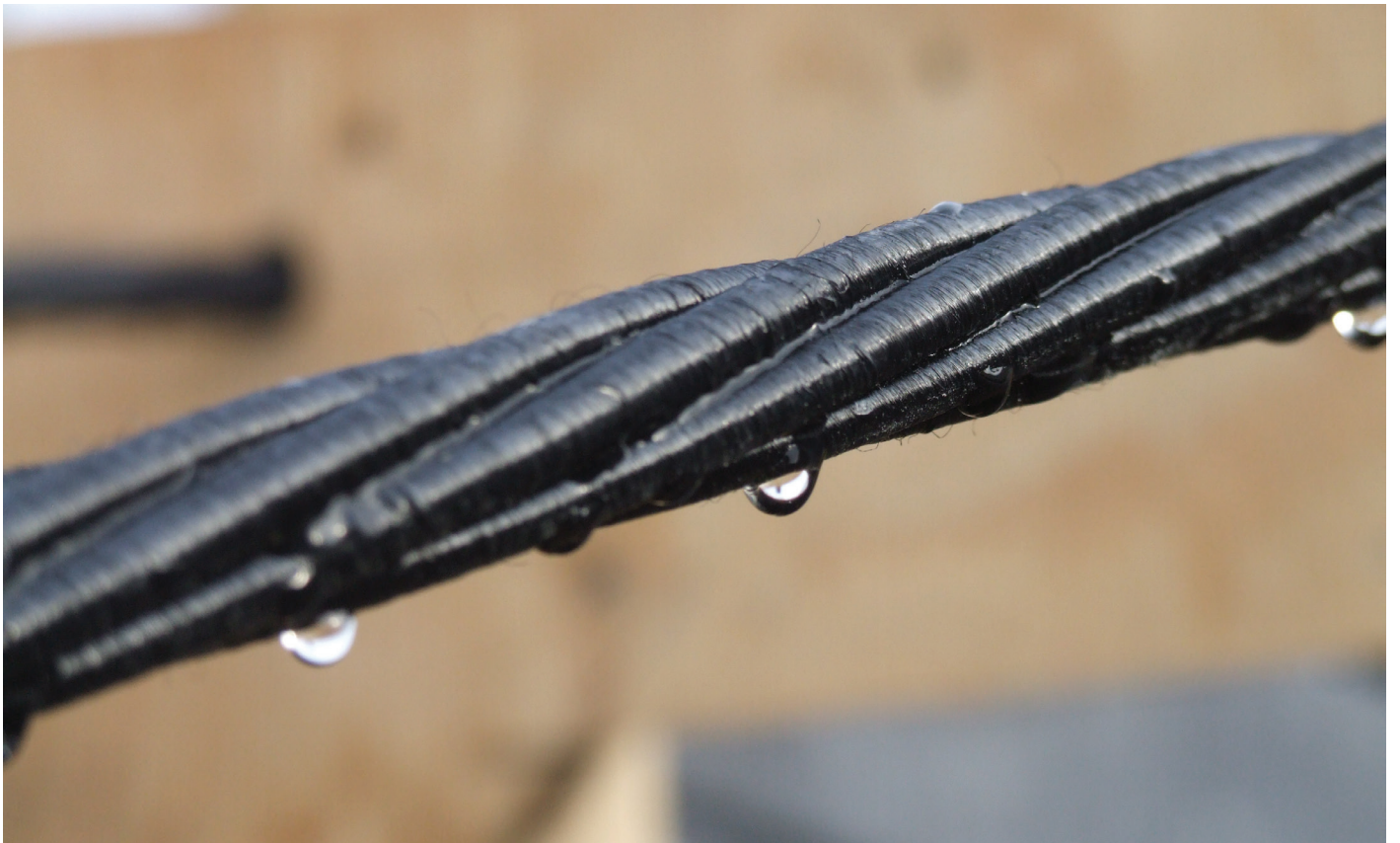
▶ If the CFRP design is selected, the CFRP reinforced beams or piles will be corrosion free. This photograph shows a close-up images of the CFRP strand that was taken at a fabricator's facility in the morning after a rain storm as they made beams as part of an earlier VDOT project.
