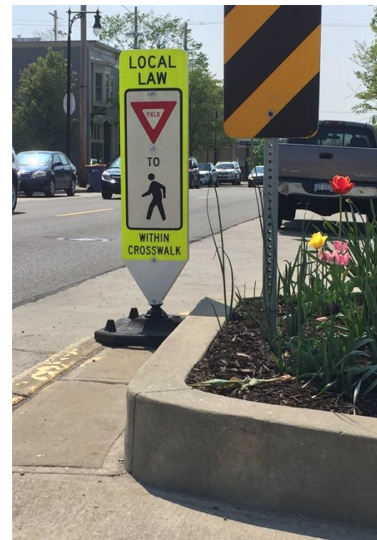
Figures 2a-c. Figure 2a (above left) shows an R1-6 sign installed on a removable curb base. Figure 2b (middle) shows a flexible delineator installation. Figure 2c (above right) shows an R1-6 sign mounted on a flush mounted base.
