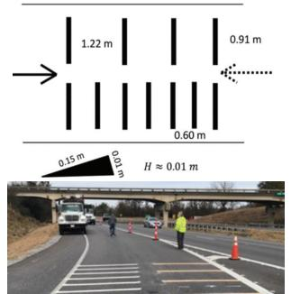
• Caltrans DRISI, Bosch Mobility Solutions, and UC Davis have been testing a Bosch cloud-based mobile device wrong way driver detection and alert system on California state highways.
