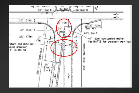
From 8° angle between ramps to 11° angle.
