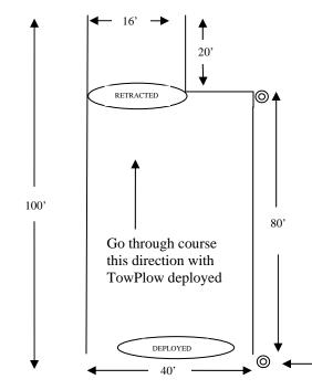
Object of this course is speed control, recognizing obstacle in the way, timing and control of the TowPlow.
