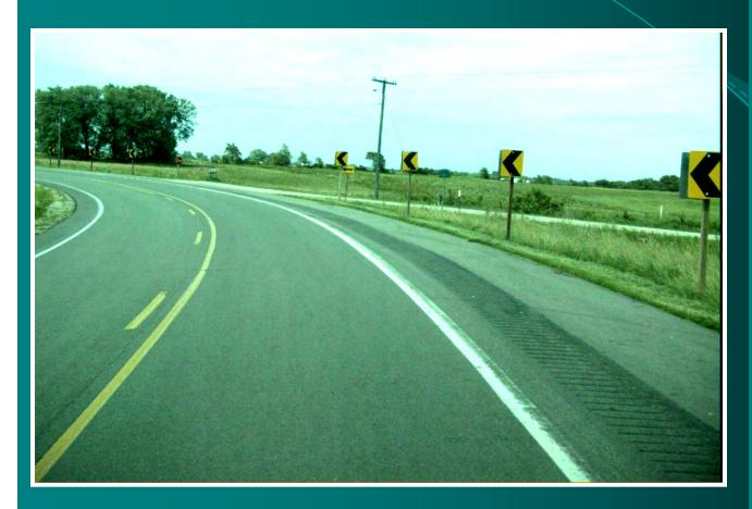
Super elevation: add or correct Pave shoulders: outside & inside Flatten outside slope Remove objects outside curve Delineate, chevron, RPM's, ball bank advisory
