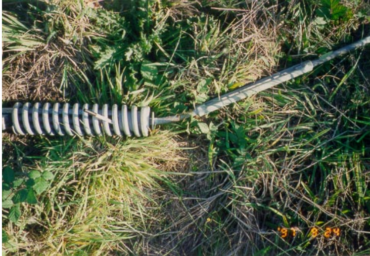
Figure 3.10: Energy dissipation-spring cable turnbuckle deformation
