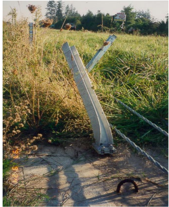
Figure 3.9: Energy dissipation-weak-post bending
