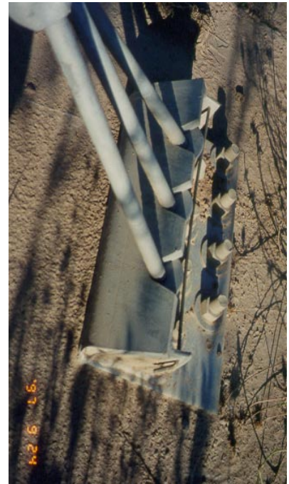
Figure 2.6: Breakaway anchor angle
