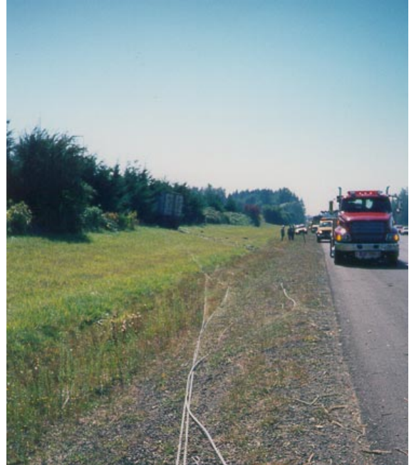
Figure 3.3: Semi-truck pulled barrier cables across northbound lanes
