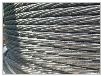
Carbon Fiber Composite Cable (CFCC)
