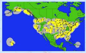
12/02 - Approximately 85% the contiguous 48 states receive correction signal from at least one NDGPS transmitting site; 12/03- All contiguous 48 states expected to receive the signal from at least two transmitting sites.
