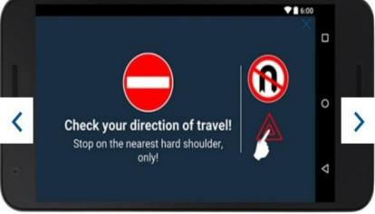
Bosch's software transmits regular, anonymized position data to a server in a central computing center. The server contains a web-based database of maps and corresponding permitted directions of travel. When the server detects a conflict in travel direction, the wrong-way driver, and all proximate networked road users, automatically receive a warning presented through the third-party app 2.
