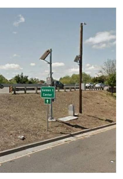
The newly installed directional sign to the Golden 1 Center blocked the rearfacing radar detector of the TAPCO system at US 50 and 16th Street. (The UC Davis detection system can be seen on the wood pole in the background.)
