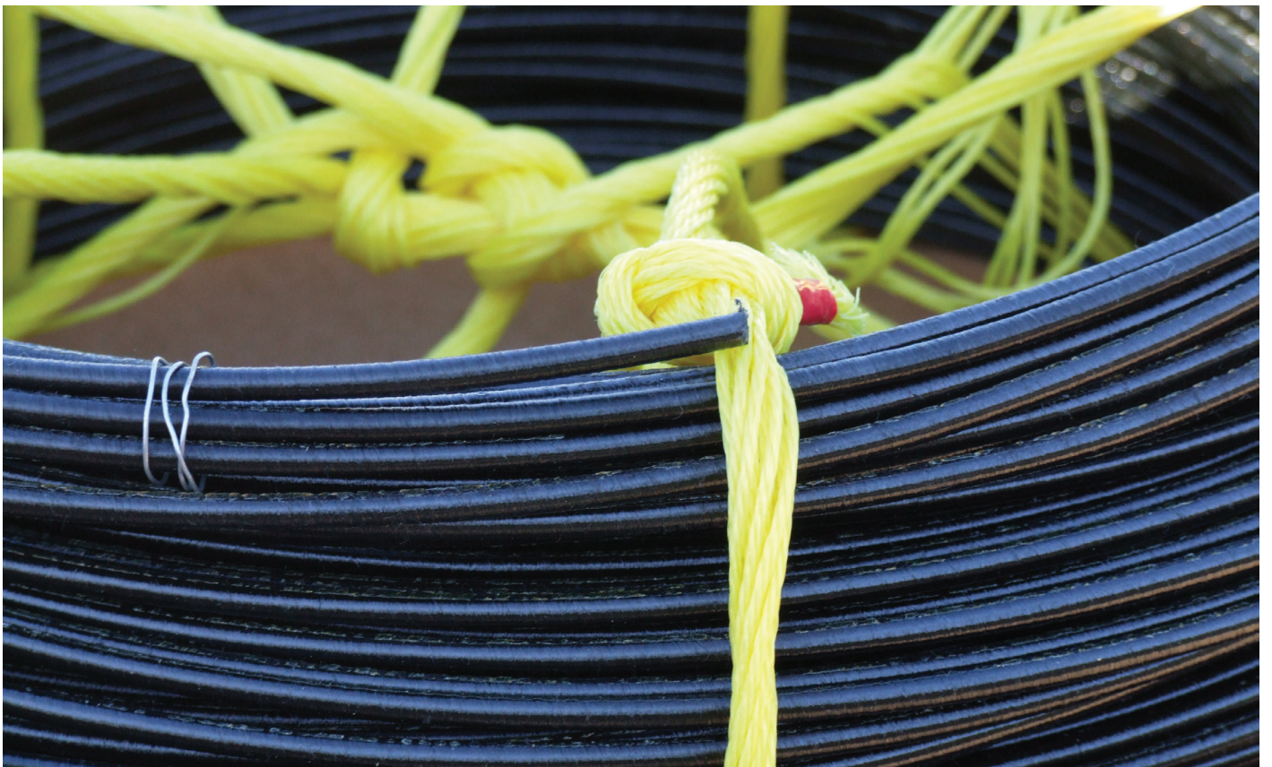
▶ This photograph shows as example from an earlier VDOT project of what the preformed CFRP spiral looked like before it was untied and the spirals properly spaced out along the length of a precast concrete CFRP reinforced pile. These piles are corrosion free.
