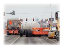
Operators have found that in large multilane intersections retracting the Tow Plow enough to clear traffic and obstacles allows for a large area of the intersection to be cleared in one pass. Good judgment and communication with operators of single front plow trucks may be necessary to provide efficient clearing of large multilane intersections.
