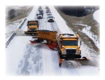
results while reducing snow removal costs for equipment, fuel and labor. The Tow Plow is a large piece of equipment and requires a skilled operator. Proper training, knowledge and experience are essential for an operator to maximize the Tow Plow's benefits in snow removal operations.
