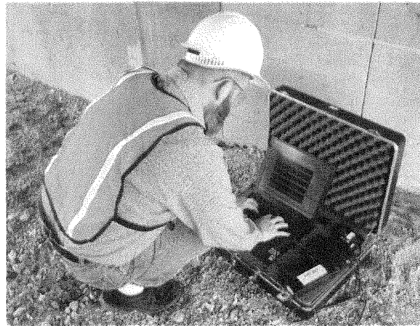
The DSRM (Laser Profilometer) is a field (or laboratory) instrument to measure concrete surface roughness.
