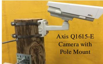
The AHMCT researchers developed and installed zone-triggered video-based site monitoring (VBSM) systems at 8 off-ramps on which active detection and alerting systems were later installed.
