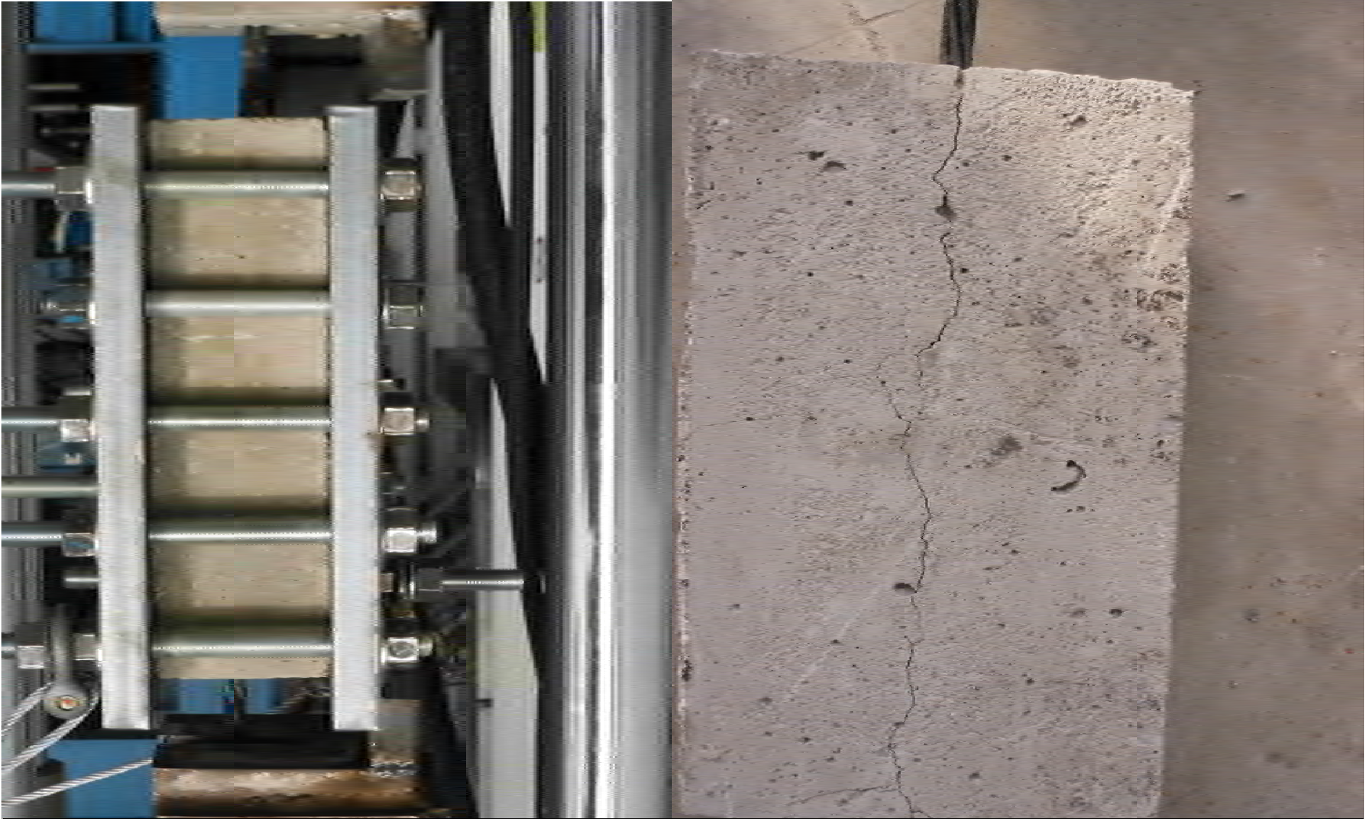
Loading and failure of specimens with lateral confinement (4"×8"×15")
