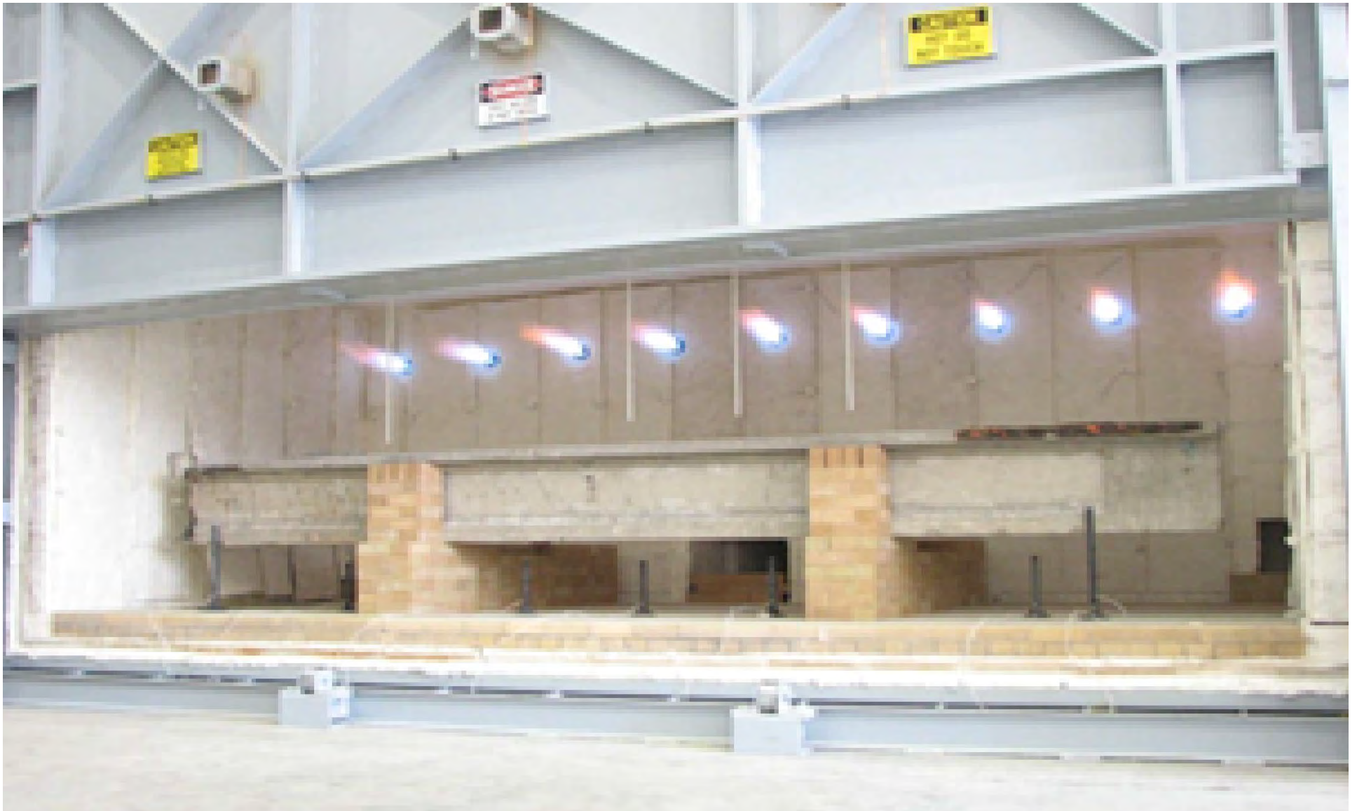
Beam testing under three-point load setup in fire chamber
