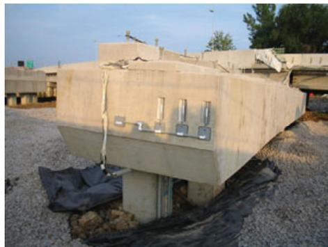
An instrumented concrete pile and cap at the Woodrow Wilson Bridge outside of Washington, DC. The instrumentation system is collecting strain and acceleration data
