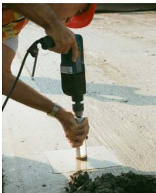
AVA specimens are collected by vibrating a wire cage into fresh concrete using a percussion drill. The mortar fills the cage and a syringe captures a mortar sample.
