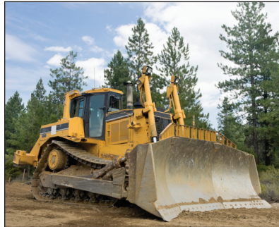
AMG computer software guides construction equipment such as this bulldozer for improved speed and accuracy.
