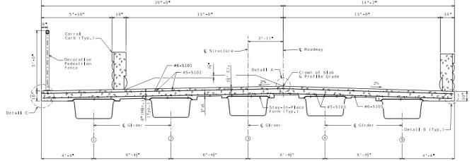
SECTION THRU SLAB (Looking Upstation)
