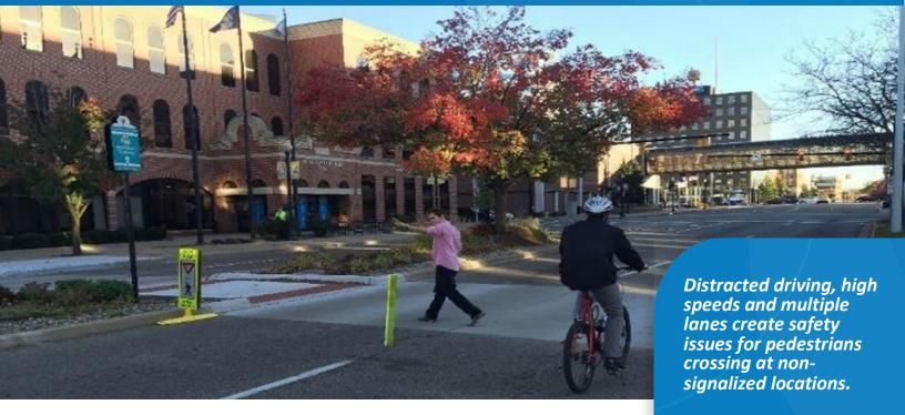
The Pedestrian Gateway Treatment can be made up of R1-6 pedestrian in-street signs installed at the curb and on all lane lines and/or R1-6 signs installed at the curb and flexible delineator posts installed on lane lines. Appropriate installation locations include intersections and midblock crosswalks on roads with speed limits of 35 mph or less. Because the treatment components are simple and adaptable, the treatment can be used in a variety of roadway configurations including one- and
