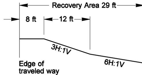
$$\begin{aligned} \text{Recovery area} &= (\text{shoulder width}) + (\text{horizontal distance}) \\ &+ (\text{Design Clear Zone distance} - \text{shoulder width}) \\ &= 8 + 12 + (17-8) \\ &= 29 \text{ feet} \end{aligned}$$
