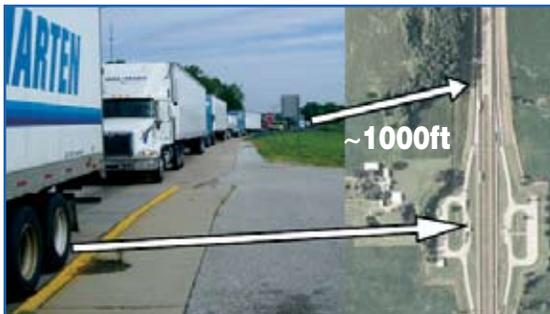
Indiana's Seymour Weigh Station, May 9, 2006: Backups like this make the case for VWIM; it developed 10 minutes after the scale house opened. Trucks are forced to bypass because the station weighing them can't handle the throughput.
