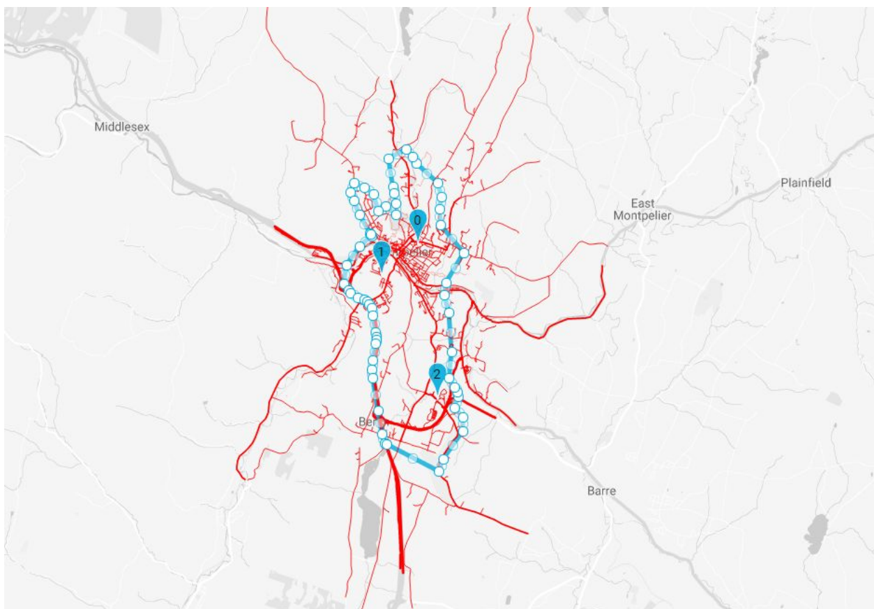
Screenshot of Via's simulation tool, showing a potential microtransit zone (outlined in blue) and three "terminals," which are discussed below. The red lines show roads, with different widths representing different road classifications, each with a different traffic speed.
