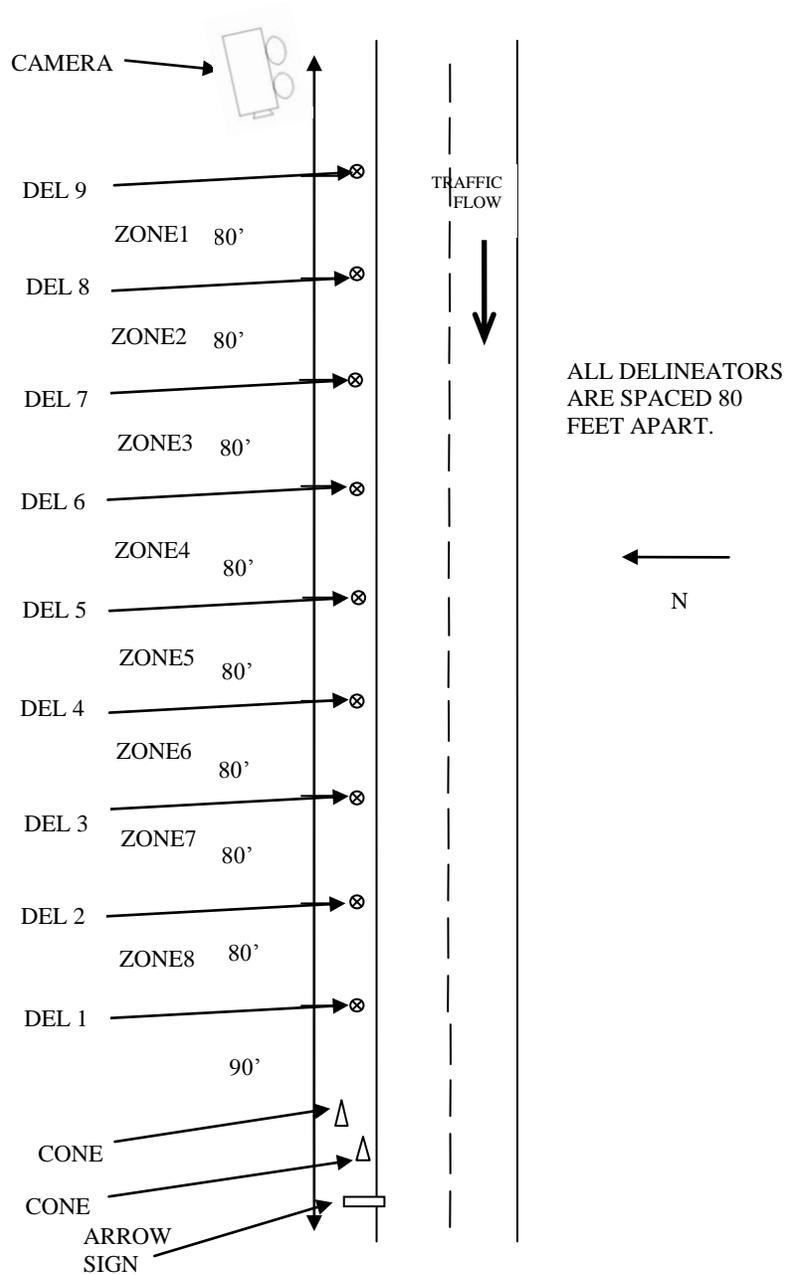
**FIGURE 6** Layout of delineator setting in the field.
