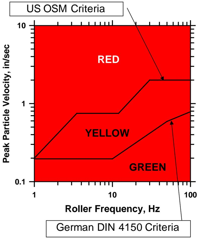
Figure 1 FDOT Adopted Vibration Threshold Criteria
