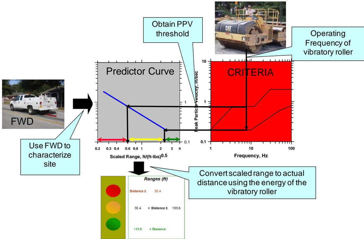
**Figure 2 Overall Vibration Analysis Procedure**
