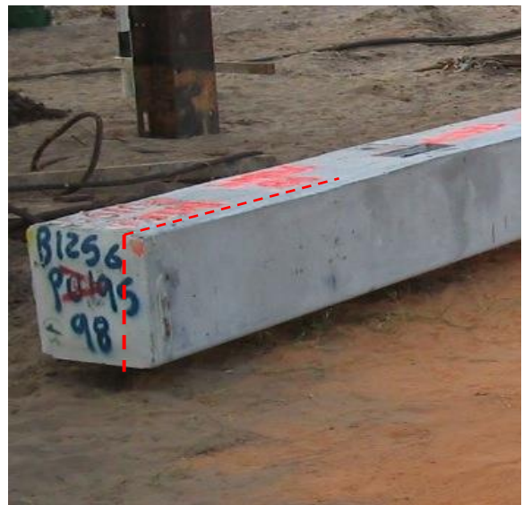
Figure 1: Orientation of vertical cracking
