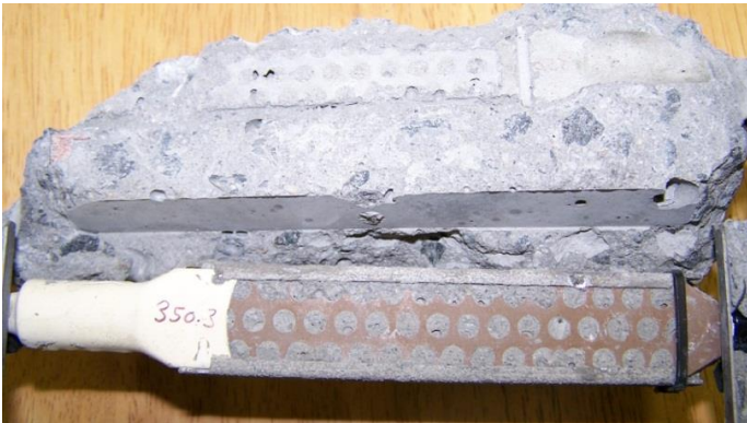
Figure 8: Another embedment strain gauge extraction, now showing close-up of bonding effectiveness of waffle pattern. Note the negative image of the pattern visible in loose piece of concrete above (rotated)
