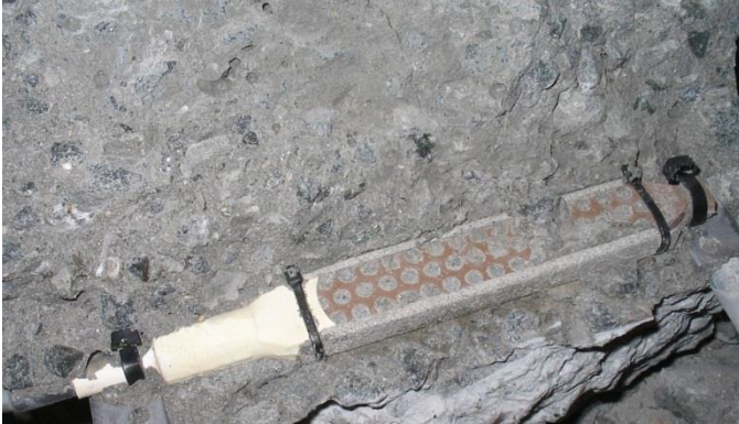
Figure 7: Embedment strain gauge manually chiseled out of solid 24" PSC pile end to show encapsulation effectiveness and material bonding. Note the lack of any visible material voids in surrounding concrete
