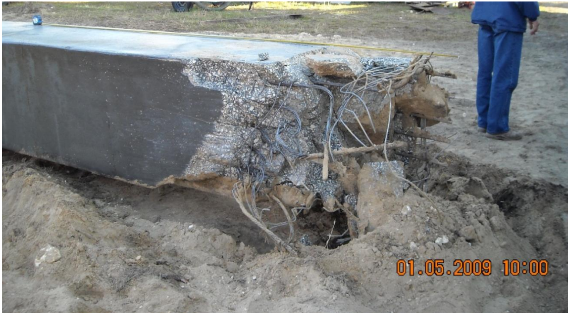
Figure 6: Example of material disturbance. Driven pile referenced from data above after extraction. Vertical cracks extend 10 feet up from the pile tip as noted by the visible ends of the tape measure. The tip instrumentation located in a segmented mass within pile core remained operational.
