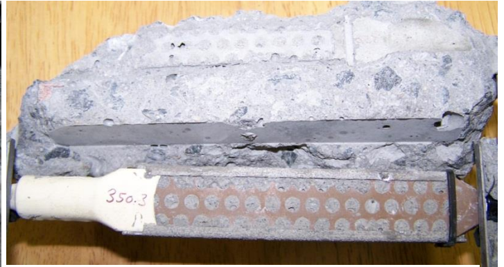
Figure 8: Another embedment strain gauge extraction, now showing close-up of bonding effectiveness of waffle pattern. Note the negative image of the pattern visible in loose piece of concrete above (rotated)
