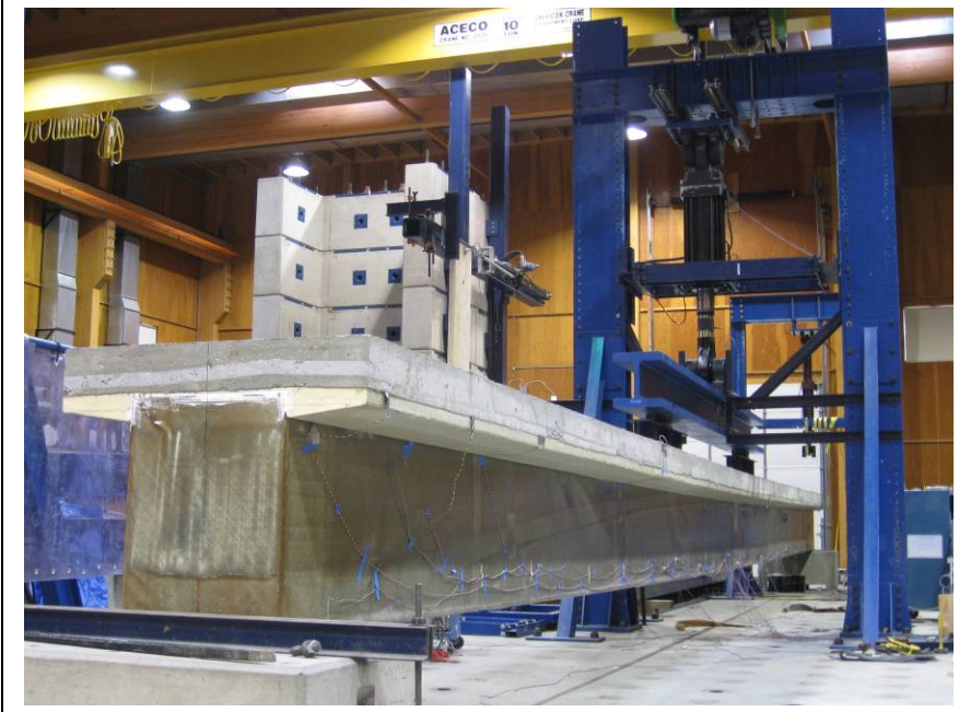
Fig 2 – April 2009 - Prototype Test Beam for Knickerbocker Bridge in Boothbay, ME. 33-inch deep HCB with 7-inch deck, 70-foot long was load tested to 2M cycles with ultimate capacity having: Operating Rating Factor = 3.48 Inventory Rating Factor = 2.68
