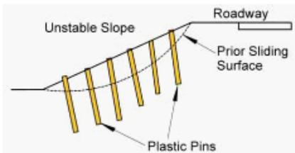
Reinforcement of unstable slope with recycled plastic pins
