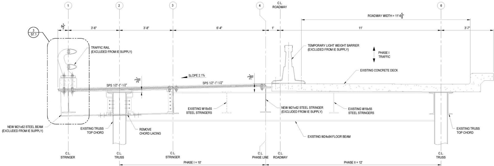
1 TYPICAL BRIDGE CROSS SECTION (CONSTRUCTION PHASE I)
