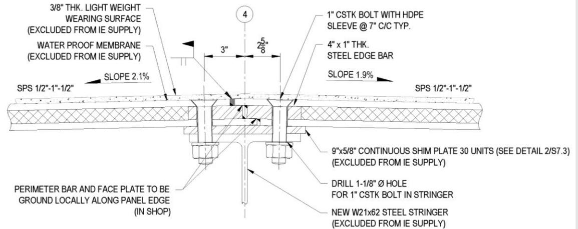
1 TYPICAL SPS PANEL CONNECTION AT BRIDGE CROWN
