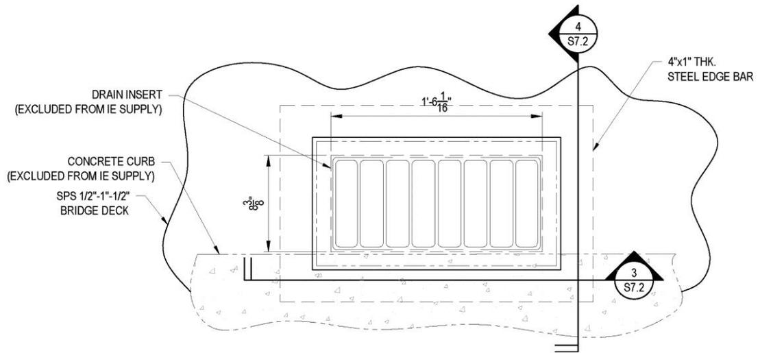
2 TYPICAL PLAN VIEW OF DECK DRAIN
