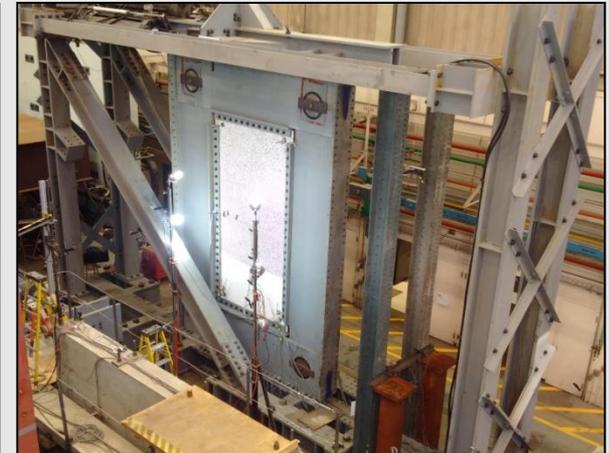
**Full Scale In-Plane Shear Test**
